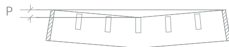
Deviations for concave P max. = 1/200 of the length for dimensions > 600 \text{ mm} ; max. 8 mm for dimensions smaller than 600 mm; max. 3 mm
